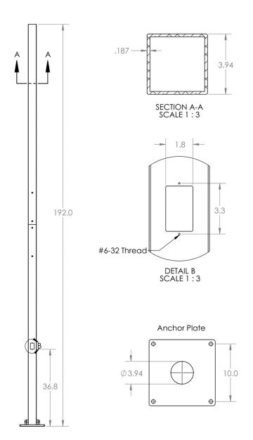
**Pole:** Square profile extrusions made from high-strength Aluminum 6061 T6. The light pole assembly is rust proof. **Pole Top:** Designed to accommodate slip-fit tenons and drill mounted tenons.
